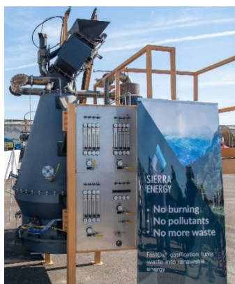
Left: First-generation Sierra Energy's FastOX™ system turns waste into hydrogen to power zero-emission trains. | Right: Ribbon Cutting group | Photo Credit: California Department of Transportation
